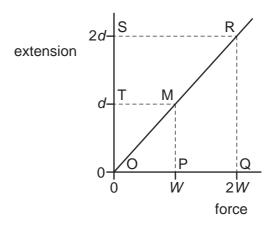
Initially a force W gives an extension d. The force is then increased to 2W. This increases the extension to 2d.
