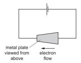
Electrons move clockwise around the circuit.
